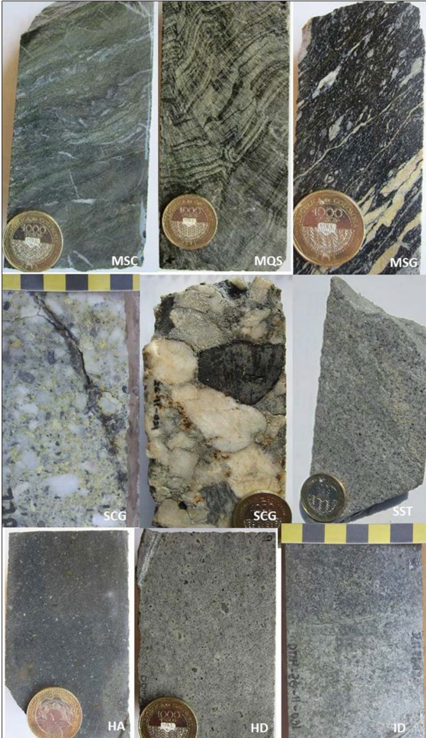
Notes: Top row: MSC, Chlorite schist; MQS, Quartz sericite schist; MSG Graphite schist. Middle row: SCG Conglomerate, SST Sandstone. Bottom row: HA, Andesite porphyry; HD, Dacite porphyry; ID, Diorite. Source: IAMGOLD, 2020 and photos by S. Redwood.
